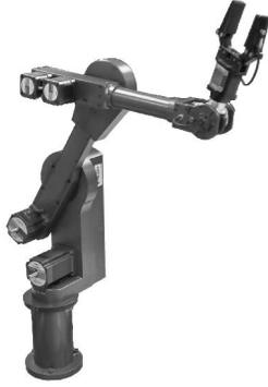
Figure 2. The PENTAXIS 5-DOF manipulator.
