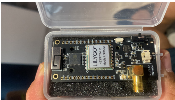
Figure 2: LILYGO TTGO LoRa32 433 MHz V1.6.1 development board.
