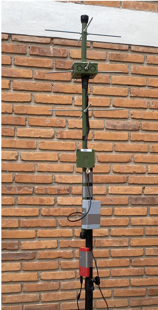
Figure 6: The whole ground station: antenna (in green), LoRa receiver system (in gray), and battery (in red).
