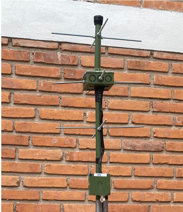
Figure 1: Turnstile antenna used for satellite telemetry reception.
