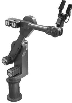
Figure 2. The PENTAXIS 5-DOF manipulator.
