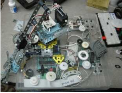
Figura 4. Implementing de two feedback potentiometers for use with the digital PID.
